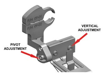
5 - When the mount is positioned as far forrward as it will go, tighten the clamp screw untill the Top and Mid Sections are slightly snug around the mirror stem. You should still be able to rotate the mount. Rotate the mount so it is parallel with the bottom of the mirror. Tighten the clamp screw untill the mount is securely attached to the mirror stem.
