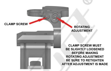
6 - Use adjustments shown to install RD to your desired position. We recommend adjusting RD as close to bottom of mirror as possible. Be sure to tighten vertical and pivot adjustment screws after adjustments are made. For Pivot adjustment, grab long arm of allen wrench for maximum leverage. You will not strip the threaded holes in the aircraft grade aluminum.
