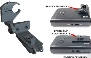
1 - Remove the socket head bolt and the existing mount from the radar. Install the spring clip adapter plate with the supplied hex key, bolt, and O-ring as shown above.
