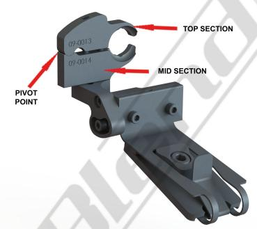
3 - Loosen the CLAMP SCREW so there is enough clearance between the TOP and MID SECTIONS to slide over the mirror stem. YOU MAY ADJUST THE MIRROR PARALELL TO THE WINDSHIELD AND SLIGHTLY UPWARD FOR EASE OF INSTALLATION.
